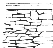
Concrete pre-cast coping.
