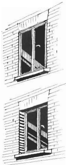
Deep window reveals as shown in the lower sketch provide better weather protection and give a sense of solidity.
