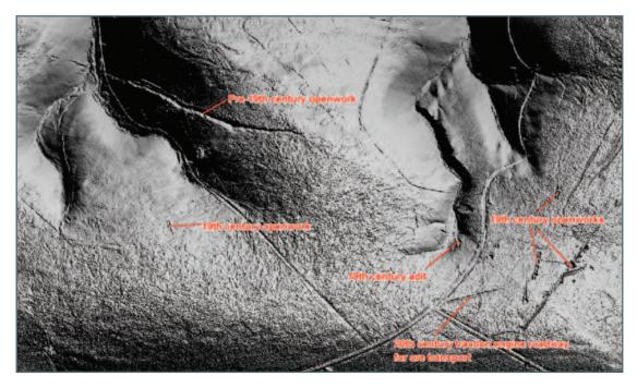
Figure 4: LiDAR digital terrain model showing the mining landscape on Burcombe and Deer Park.
